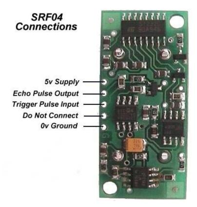
The SRF04 Timing diagram is shown below. You only need to supply a short 10uS pulse to the trigger input to
