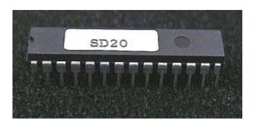
The SD20 chip is a pre-programmed PIC16F872 running at 8MHz. Position commands for up to 20 servo's are sent to the chip over the I2C bus.
