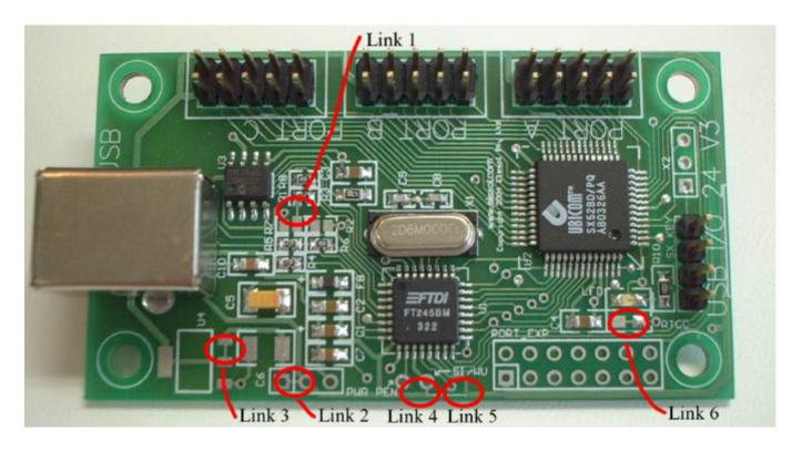
**Link 1** = remove link to use FTDI chip in Self Powered mode. Also remove components C10 and FB. Place components R2, R6, R7. Apply an external power supply (5V MAX) to pin 2 of PWR Connector.
